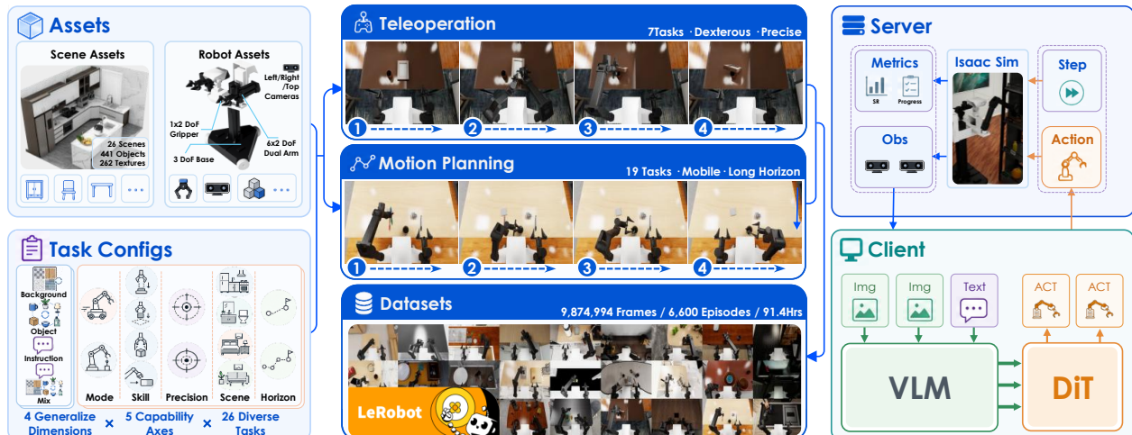
Figure 2. EBench end-to-end pipeline. Left: 26 tasks span pick-and-place, long-horizon, and dexterous-and-precise families, instantiated on shared scene and robot assets. Middle, two-track synthesis: dexterous-and-precise demonstrations are collected via human teleoperation (top); mobile and long-horizon trajectories are generated by motion planning from key-frame end-effector poses fed to cuRobo (bottom). Right: EBench is evaluated through a client–server protocol. The IsaacSim-backed server returns observations and a step signal, and VLA or WAM clients (e.g. a VLM with a DiT action head) emit actions in response.
